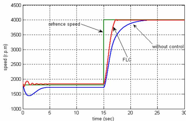
Fig. 10. Engine speed response using the FLC.
