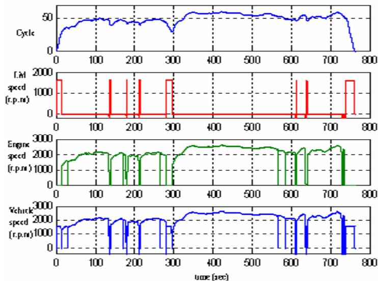
Fig. 12. Various speeds of PHEV with HY
