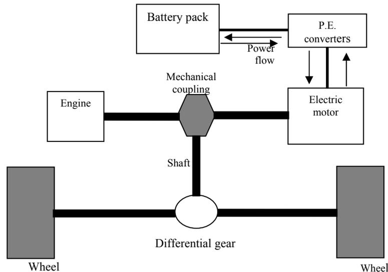
Fig.1. Parallel hybrid electric vehicles.
