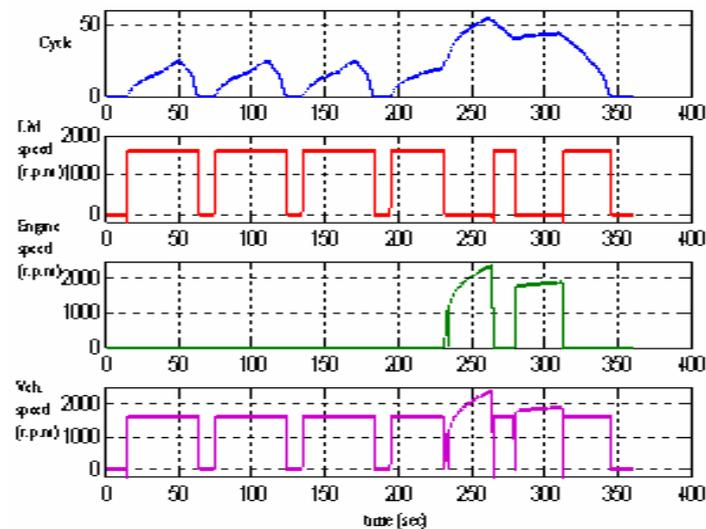
Fig. 11. Various speeds of PHEV with SFUD road cycle.
