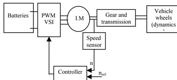
Fig.2. Block diagram of IM drives system.
