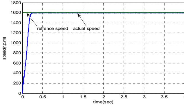
Fig.5. Speed response of IM using FLC.
