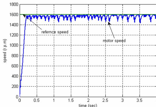
Fig.4. Speed response using PI controller.
