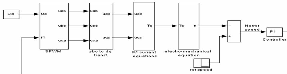
Fig. 3. Simulation block diagram of IM drive system.
