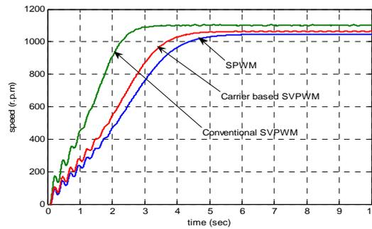
Fig. 9. Motor speed transient response of the three different PWM techniques.
