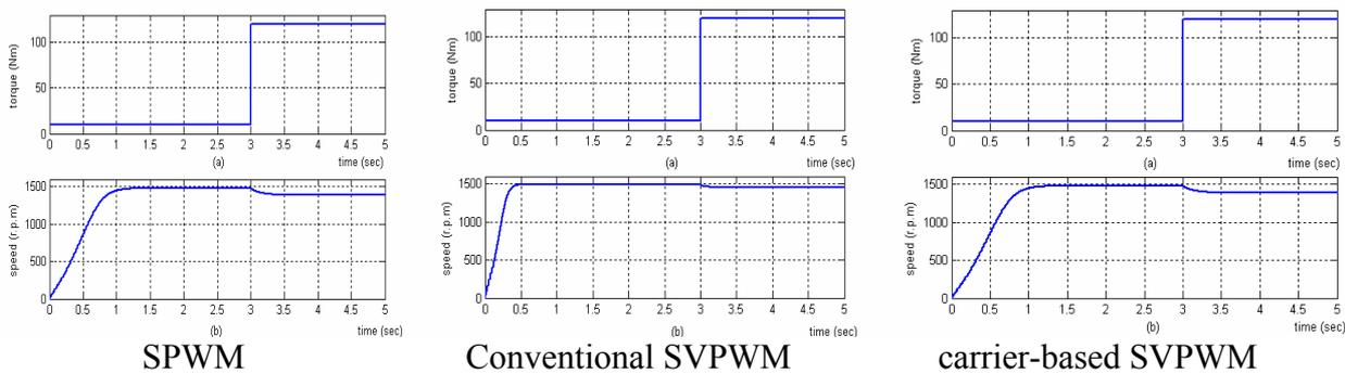
Fig. 7. System performance under varying the load torque
