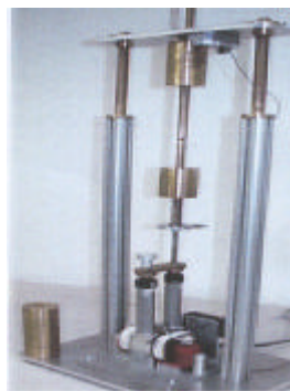
Figure 5: Robust pre-production type of MRF-based shock damper
