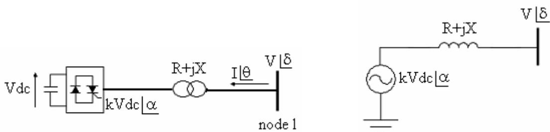
Fig.1 : STATCOM and its equivalent circuit
