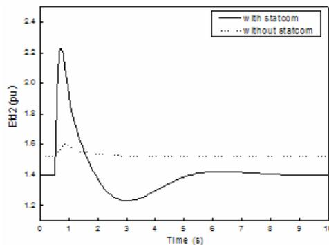
Fig.15: generator 2 excitation voltage
