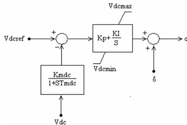
Fig.5: STATCOM amplitude control block diagram
