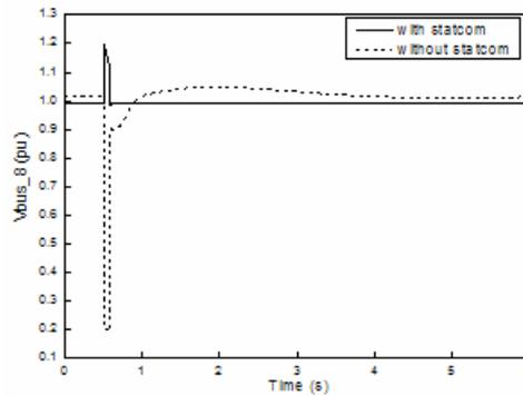
Fig.11: voltage at bus 8
