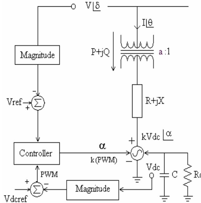
Fig.3 : Transient stability model of the STATCOM
