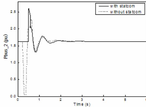
Fig.14: generator 2 active power
