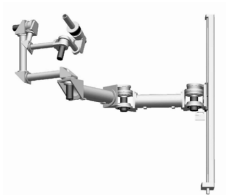
Fig. 2 Model of 7 DOF redundant manipulator
