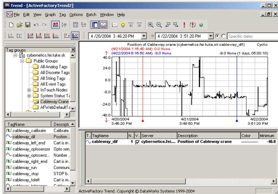
Fig. 6 Active Factory trend – analysis tools of data from InSQL database
