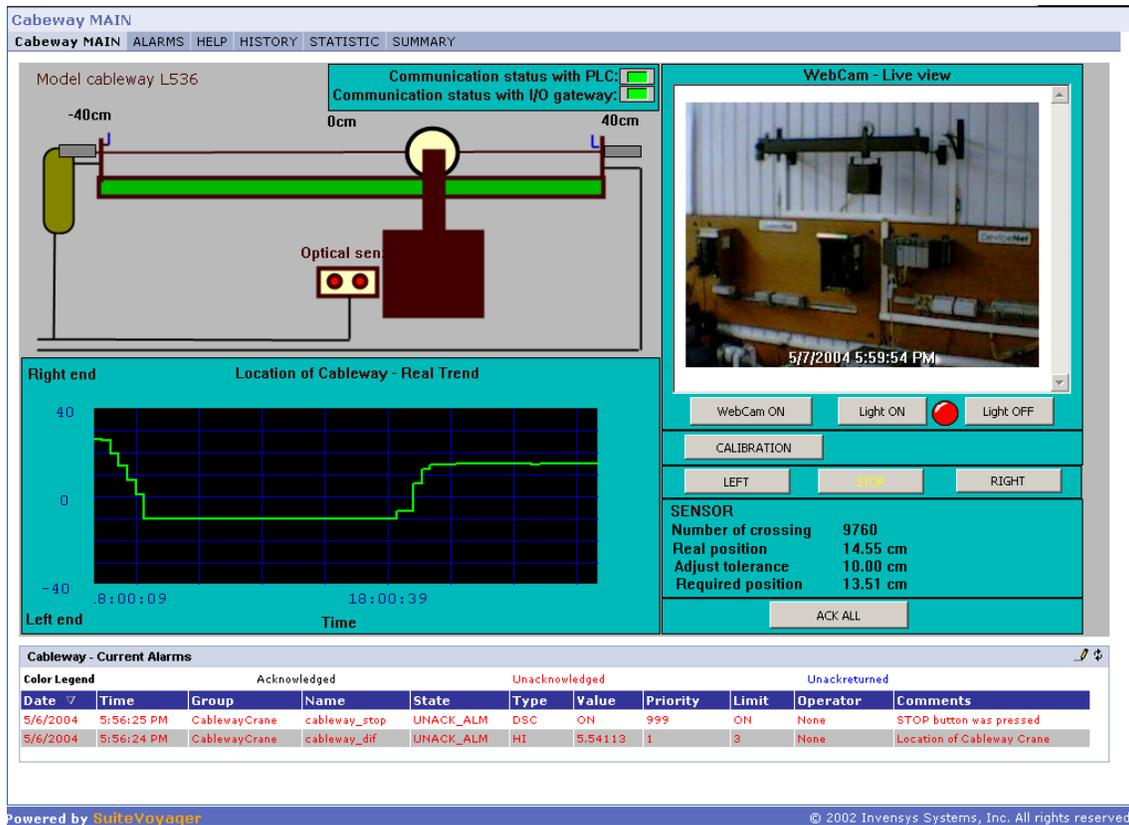
Fig. 5 HMI for cableway and summary alarms from InSQL database
